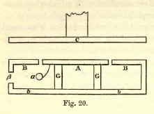
surface consists of two parts, a disk A, and a broad ring BB surrounding the disk, separated from it by a very small interval all round, just sufficient to prevent sparks passing. The upper surface of the disk is accurately in the same plane with that of the guard-ring. The disk is
