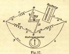
current through the galvanometer when O and B are connected by a conductor of no sensible resistance, and  $y_1$  the current when O and B are completely disconnected.
