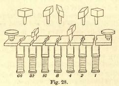
The electrodes consist of stout brass plates, so arranged on the outside of the box that by inserting a brass plug or wedge between
