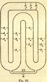
Now let the piston be moved from  $P_0$  to  $P_1$ , a distance a. Then, since the sections of all the tubes are equal, the level of the mercury in A and C will rise a distance a, or to  $A_1$  and  $C_1$ , and the mercury in B and D will sink an equal distance a, or to  $B_1$  and  $D_1$ .
