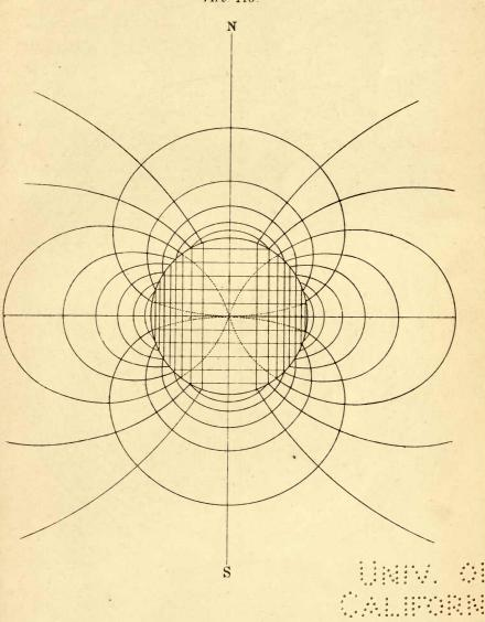
Lines of Force and Equipolential Surfaces in a diametral section of a spherical Surface in which the superficial density is a harmonic of the first degree.
