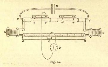
352.] The conductors to be tested are arranged in the manner already described, with the connexions as well made as possible, and it is required to compare the resistance between the marks SS' on the first conductor with the resistance between the marks T'T on the second.
